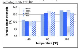
Tensile shear strength Al/Al sand- blasted at temperature related to the initial value at room temperature measured at temperature according to DIN EN 1465
