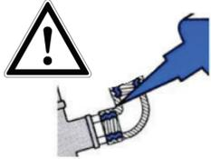
All metal to metal connections must be glued together with Loctite® 243™ (Art. No. 110278).
