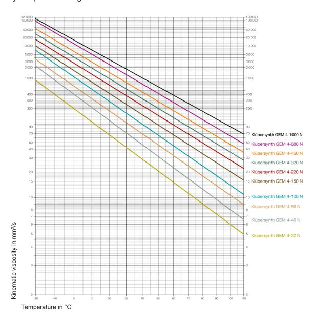
Synthetic high-performance gear and multipurpose oil with KlüberComp Lube Technology
